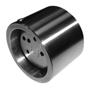
The MD Series SA3 switchgear adapter interlock has a 5/16" (8mm) square, 3/8" (9.5mm) long shaft that is controlled by the robust MD Series key. The SA3 is attached to the interlock provisions by way of (4) 10-32 tapped holes in the bottom of the lock cylinder. The interlock can be ordered with the shaft rotating clockwise or counterclockwise. Multiple degrees of rotation are available also.
